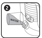
Slowly pour clean water into the machine's solution container.
