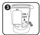
Turn ON the machine for 3 minutes, allow the machine to self-clean the inside. (This prevents the inside tubes and pump from clogging up.)
