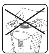
Never lift the machine by the rotating rings. This will damage the
