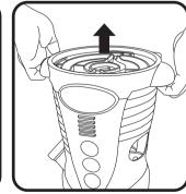
Always lift the machine by the two handles on the side.
